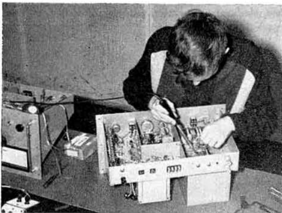
Wiring up the a.m. transmitter after a modification due to lack of drive.
